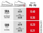
SOLE **PU / PU ESD-PLUS SRC** Double density PU sole, Outer- and in-between sole with ESD
